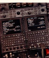
All Beechjet cabins are hits with passengers, but the 400XT's big news is up front, where Nextant provides FADEC engine controls (below), dual FMSs (below left), and Rockwell Collins Pro Line 21 avionics suite (bottom).
